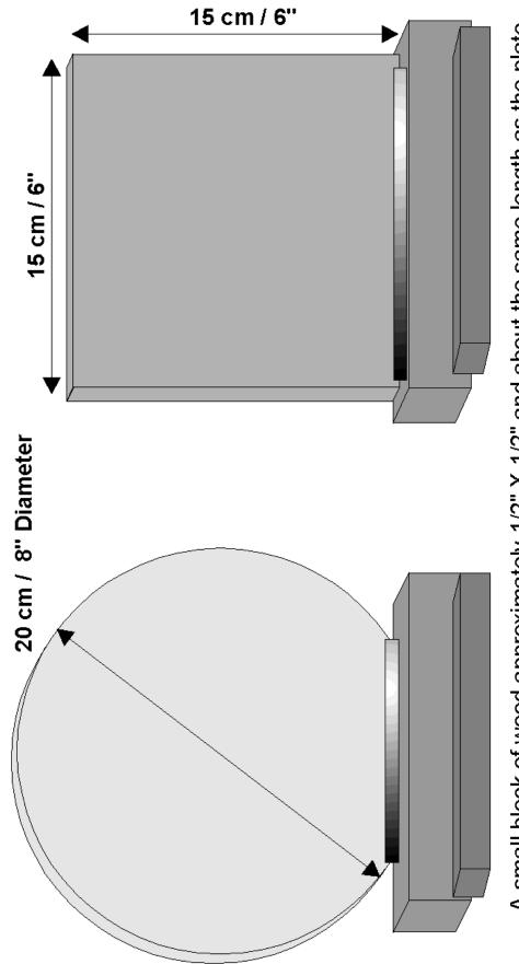
A small block of wood approximately 1/2" X 1/2" and about the same length as the plate base, is affixed in "front" of the base to prevent the plate from turning when hit.
